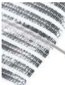
Figure.8 Energy net that is used from the outside part of a greenhouse and that can be rolled [3].
