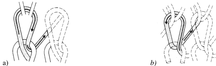
Fig. 6. a) The open-lap i b) The closed-lap loop at the formation of knitwear [2]
