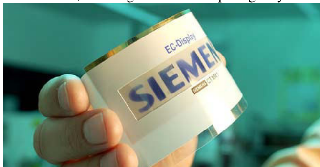
Figure 3. A flexible electrochromic display, as developed by Siemens
