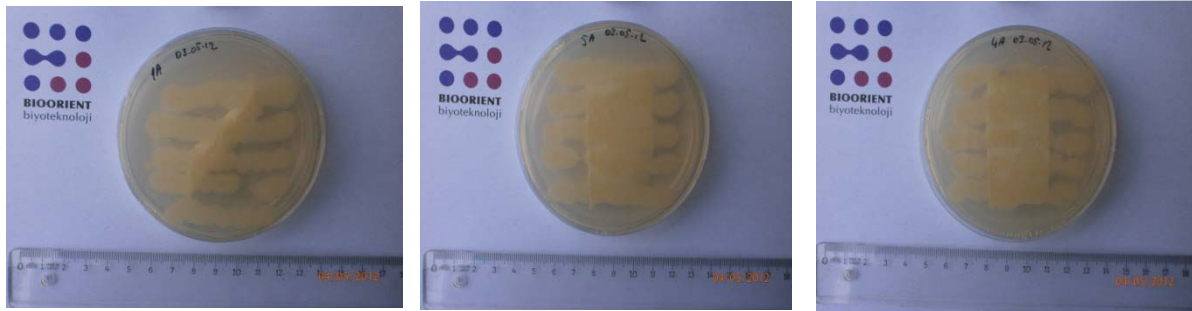
Figure 2. Antibacterial test results for fabric samples according to the AATCC 147 Standard Test Method: a) 1011 b) 3011 c) 3033
