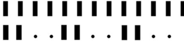
Figure. 2. Diagram of needle threading: first row shows that all sets of needles are threaded, in second row two sets are alternately threaded.
