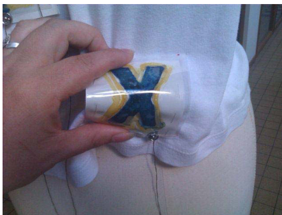
Figure 9. Showing the flexible nature of the electrochromic device
