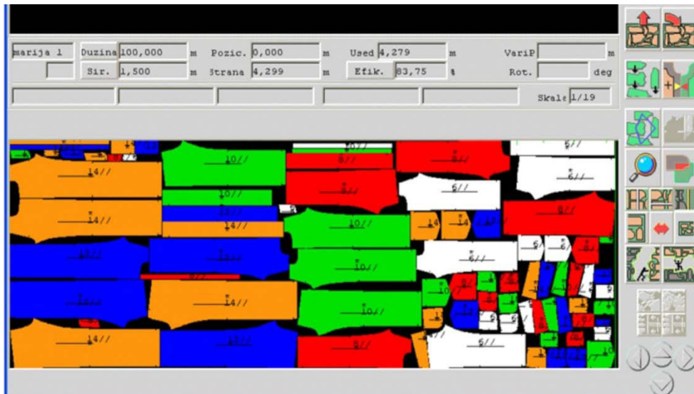
Figure 2. Cutting pattern of model M1 where the cutting parts are nested into two directions
