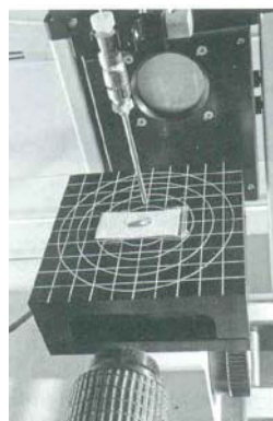
Figure 1. The device for testing moisture absorption and transport of textile materials
