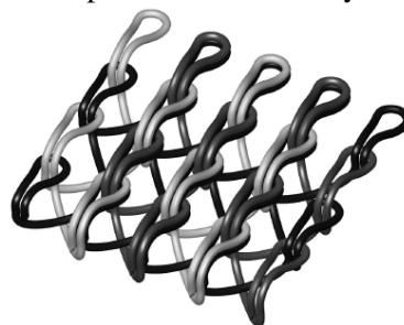
Fig. 5. Example of modelled warp knitted structure with loops from two yarns.
